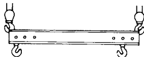
Two Hooks or Shackles can be Provided Below the Beam in Fixed Position or Movable as Shown
