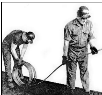
Perhaps the most common and easiest uncoiling method is to hold one end of the rope while the coil is rolled along the ground.
