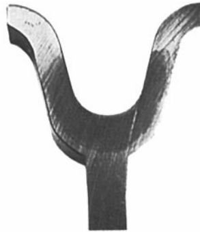
Sheave Section Cut
