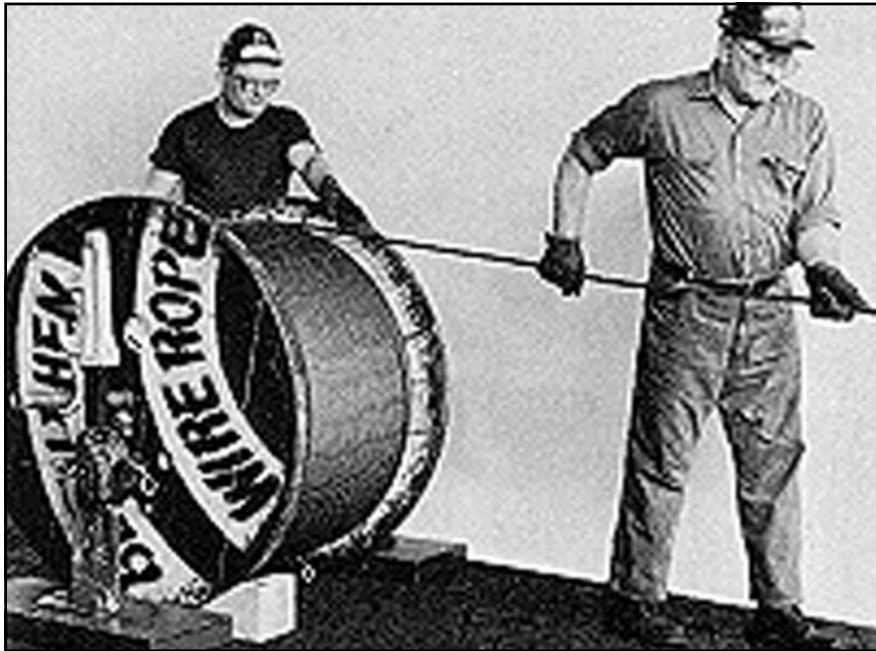
The wire rope reel is mounted on a shaft supported by jacks. This permits the reel to rotate freely, and the rope can be unwound either manually or by a powered mechanism.
